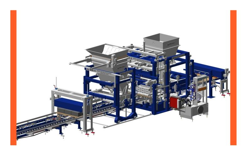
Machines of the BM 9 are equiped - with the proven technology. The production area is available from 9 to 12 blocks per Cycle. The high quality results derived from advanced vibration technology and height control precision are now possible across a wide range of products, from 40mm pavers to 200 mm high wall units.
